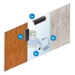
The client-side loudspeaker should be mounted at least 1 m (40 in) away from the client-side microphone and, if possible, should not face the microphone directly because this leads to an echo of the operator's voice on the client side. It is recommended to choose one of the following mounting versions:
