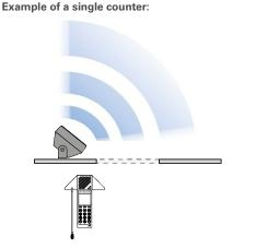
In this setup, the voice of the operator is audible in the entire area in front of the counter.
