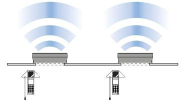
Example of how to use the directivity of a loudspeaker line array (e.g. AL 10-16) for addressing individual queues separately via horizontal mounting above the counter.
