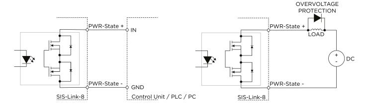
It is recommended to integrate external overvoltage protection (especially for inductive loads).
